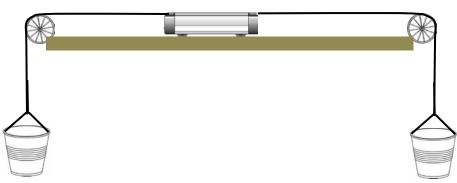
When objects, such as sugar cubes, are added to the cups, they will pull downward on the string. The string, in turn, will apply a force to the cart. When the cart is released it will be free to move and you will be able to see what effect the combination of the two forces acting on the cart has.
